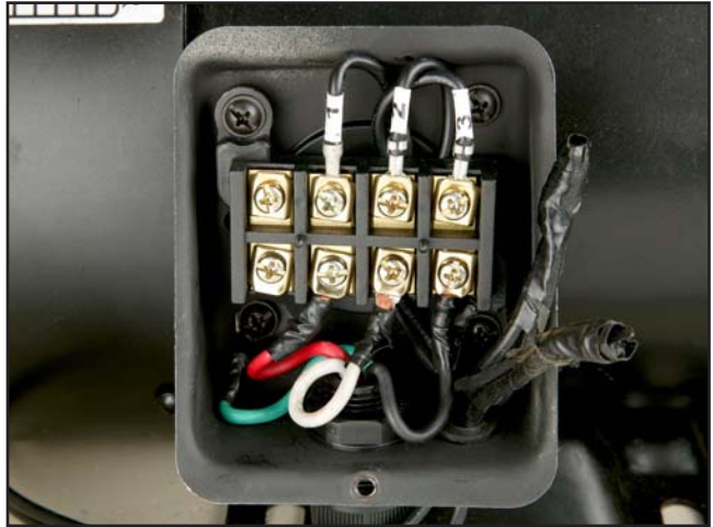
Figure 66. Motor junction box wiring.
